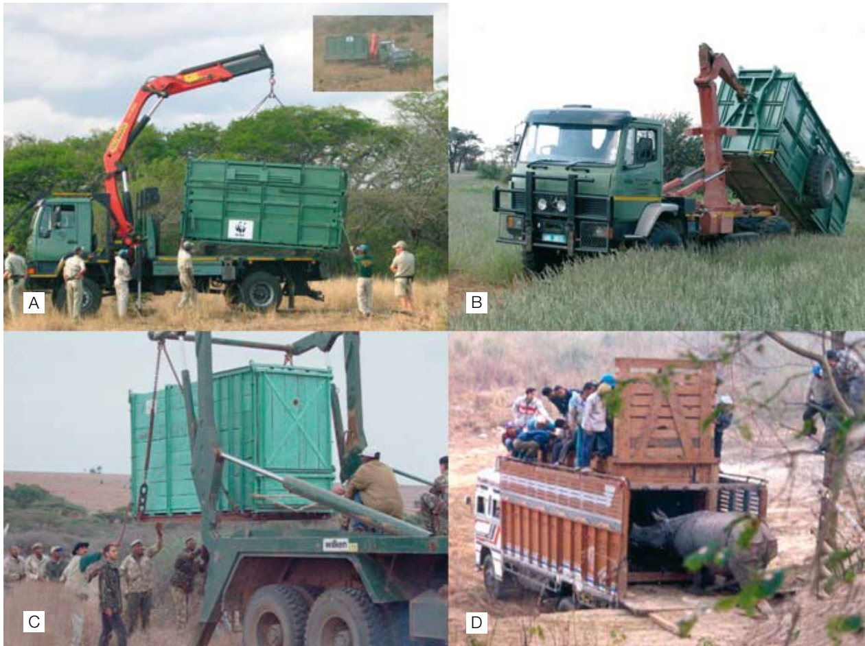
Figure 28. (A) Crane arm being used to lift crate with rhino off rhino truck in KwaZulu-Natal, South Africa; (B) Namibian Multilift system lifting crate onto truck; (C) wooden crate reinforced with angle iron being used to transport wild caught black rhino to bomas in Kenya being hydraulically lifted using the “Hannibal” system onto a specially designed rhino transporter; (D) release of greater one-horned rhino from a crate loaded onto standard truck in Nepal (Photo credits A: WWF/EKZNW BREP, B: Mark Jago, C: Rajan Amin ZSL/KWS and D: NTNC).
