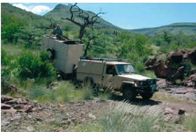
Figure 29. A number of low-cost systems have been developed and are used in some countries. The photo shows an example from Namibia, where an ordinary trailer has been modified and special crates developed to allow a black rhino and crate to be towed by a standard 4x4 vehicle. (Photo credit: Mark Jago)
